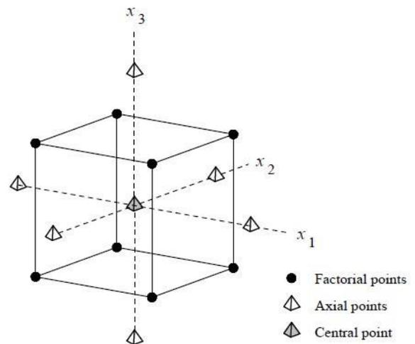
**Fig 3.1:** CCD showing 8 factorial points, 6 axial points and 6 center points used for experimentation.
