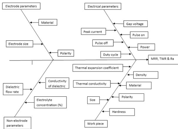
**Fig. 2.1: Process parameters of EDM**
