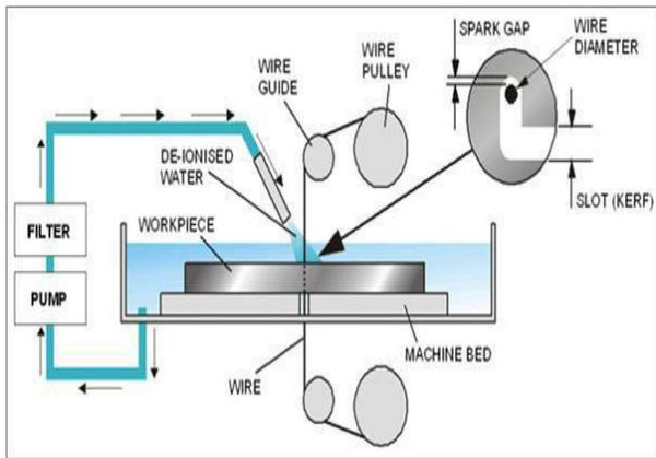
**Fig 1.1:** Schematic representation of EDM process
